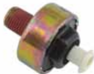
9-33501 Knock Sensor Replaces: Mercruiser 808015T Fits: MCM 262 Mag EFI, 4.3L EFI
