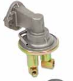
9-35401 Fuel Pump Replaces: Chrysler 3745415 Fits: 361, 400, 413, 440 V-8 Flange I.D. #: 6767, M6767
