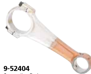
9-52400 Connecting Rod Replaces: Yamaha 650-11651-04 Fits: 15 hp
